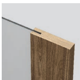
glass - door panel joint non-rebated door
